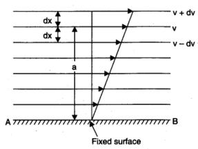
Fig. 12.01. Relative motion between different layers.
