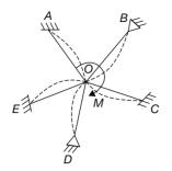
$M = M_{OA} + M_{OB} + M_{OC} + M_{OD} + M_{OE} = \text{Total applied moment}$  $S = S_{OA} + S_{OB} + S_{OC} + S_{OD} + S_{OE} = \text{Total stiffness of joint 'O'}$
