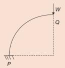
All members in the rigid-jointed frame shown are prismatic and have the same flexural stiffness *EI*. Find the magnitude of the bending moment at *Q* (In kN-m) due to the given loading. [GATE, 2013]
