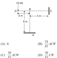
**51.** In the portal frame shown in the figure, the ratio of sway moments in column *AB* and *CD* will be equal to
