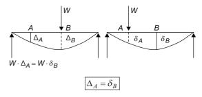
Applicable for both determinate and indeterminate structures.
