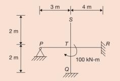
3. For the beam shown below, the value of the support moment *M* is \_\_\_\_\_ kN-m. [GATE, 2015]
