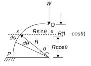
Vertical deflection at point *Q*: The bending moment at any section *X*,
