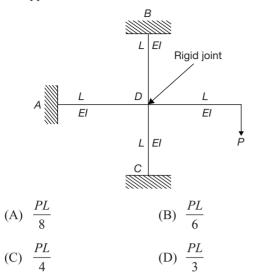
**23.** The strain energy due to bending in the cantilever beam shown in the figure is
