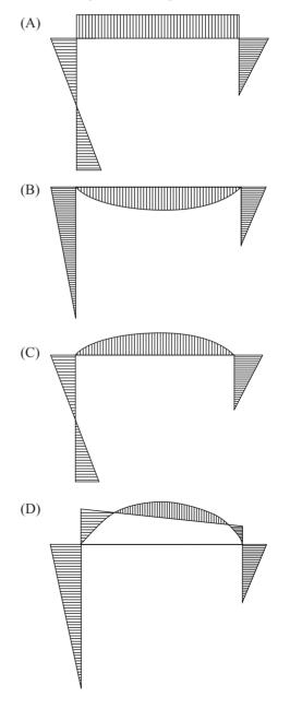
**22.** The given figure shows a frame loaded with a single concentrated load *P*. The fixed-end moment developed at support *A* will be
