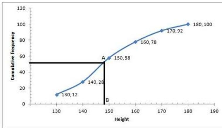
Through  $50^{\text{th}}$  term mark draw a line parallel to the x-axis which meets the curve at A. From A, draw a perpendicular to x-axis which meets it at B.
