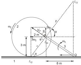
Let us assume fixed link as 1, disc as link 2 and rod as link 3. Applying Kennedy theorem:
