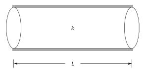
For 1-d steady state without internal heat generation heat conduction equation
