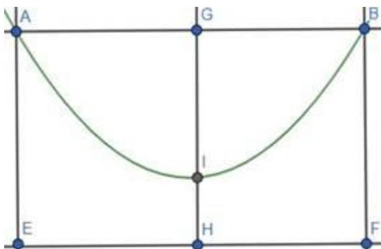
A and B are the top of the towers. AE and BF are the height of the towers. H is the center of the bridge. HI is the 5 m above from the roadway.
