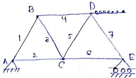
truss system = members + Pins/joints
