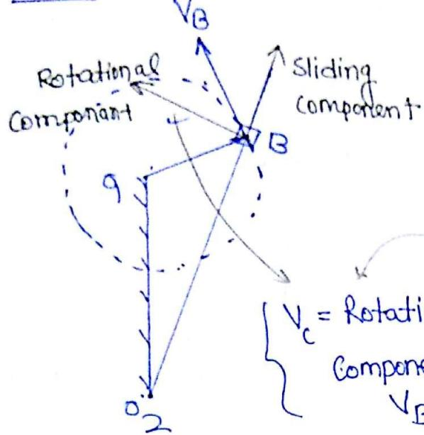
Point C:- coincident point of slider B, but on slotted bar
