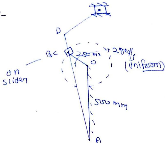
find the Angular Velocity of slotted bar when the Velocity of Ram is max.
