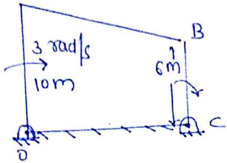
Pb 1:- The velocity diagram to the given conf. at this instant.
