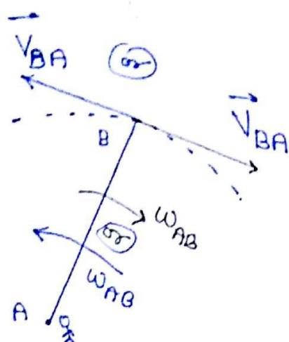
$\vec{v}_{BA}$  = The velocity of point B w.r.t. point A will be in the perp to the link AB.
