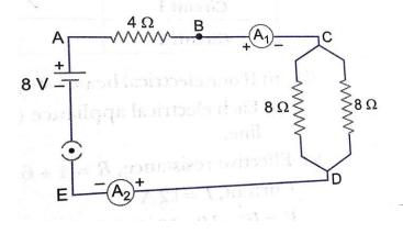
Ans. (a)  $R = \frac{R_1 R_2}{R_1 R_2} = \left(\frac{8 \times 8}{8 + 8}\right) = 4\Omega$ (b)  $I = \frac{V}{R} = \frac{8}{4 + \left(\frac{8 \times 8}{8 + 8}\right)} = \frac{8}{8} = 1A$ (c)  $V = I R = 1 \times 4 = 4V$ (d)  $P = I^2 R = I^2 \times 4 = 4W$
