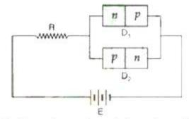
Indicate the path and direction of flow of appreciable current in the circuit.
