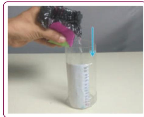
**Fig. 6.16**, Fill the cube upto the brim and measure the volume of collected water using a volume measuring beaker
