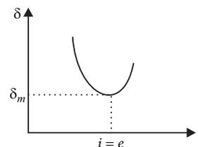
(b) At minimum deviation, the inside beam travels parallel to base of the prism.
