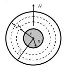
The radial rate of flow of heat through this shell in steady state
