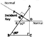
Now the normal is perpendicular to face AC of the prism, so ED will be parallel to base BC. Thus,
