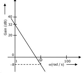
The gain  $(20 \log |G(s)|)$  is 32 dB and -8 dB at 1 rad/s and 10 rad/s respectively. The phase is negative for all  $\omega$ . The G(s) is
