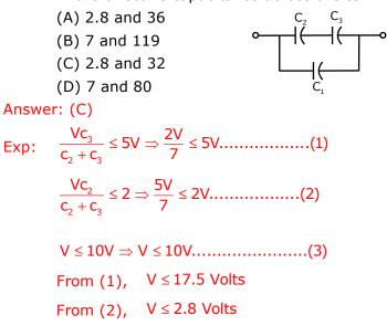
From (3),  $V \le 10$  Volts To operate Circuit safe, V should be minimum of those =2.8V  $c_{eff} = c_1 + (c_2 \parallel C_3) = 10\mu F + \frac{10}{7}\mu F = \frac{80}{7}\mu F$  $Q = c_{eff} \times 2.8V = 32\mu c$
