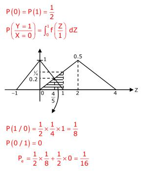
49. The optimum threshold to achieve minimum bit error rate (BER) is
