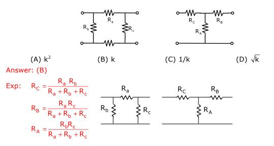
Above expression shown that if  $R_a$ ,  $R_b \& R_c$  is scaled by k,  $R_A$ ,  $R_B \& R_C$  is scaled by k only.
