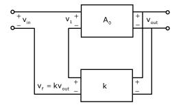
(A) The input impedance increases and output impedance decreases
