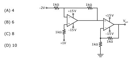
Answer: (C) Exp:  $-2V \circ \frac{1 k\Omega}{\sqrt{1 k\Omega}} \frac{1 k\Omega}{\sqrt{1 k\Omega}}$   $V_{out} = ? 1 k\Omega$   $+1V \qquad 1 k\Omega$   $V_1 = 1(1+1) - 2(-1) = 4V$  $V_{out} = 2V_1 = 8V$
