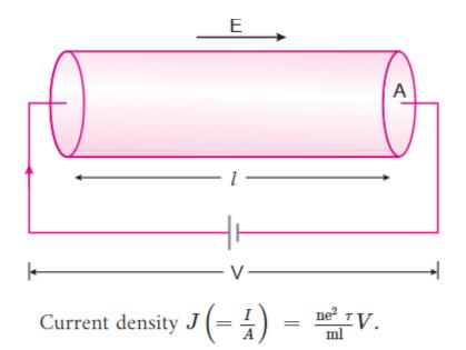
This is relation between current density J and applied potential difference V.
