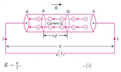
Due to this electric field, the electrons gain a drift velocity  $v_d$  opposite to direction of electric field. If q be the charge passing through the cross-section of wire in t seconds, then
