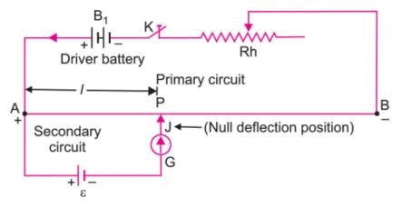
In primary circuit the rheostat (Rh) is so adjusted that the deflection in galvanometer is on one side when jockey is touched on wire at point A and on the other side when jockey is touched on wire at point B.
