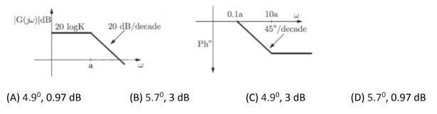
**Q.4** The asymptotic magnitude Bode plot of an open loop system G(s) with K>0 and all poles and zeroes on the s-plane is shown in the figure. It is completely symmetric about  $\omega_c$ . The minimum absolute phase angle contribution by G(s) is given by
