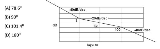
**Q.5** The open loop transfer function of a system is given by  $G(s)H(s) = \frac{100(s+100)}{s(s+10)}$  in the straight –line approximation of the Bode plot  $|G(j\omega)H(j\omega)|$  and  $\angle G(j\omega)$  at  $\omega$ =100 rad/sec are
