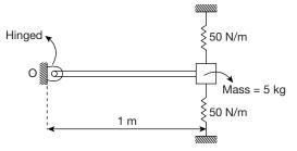
Assuming *EI* of rod = 2.67 N-m<sup>2</sup>, calculate natural frequency of the bar in (rad/sec)
