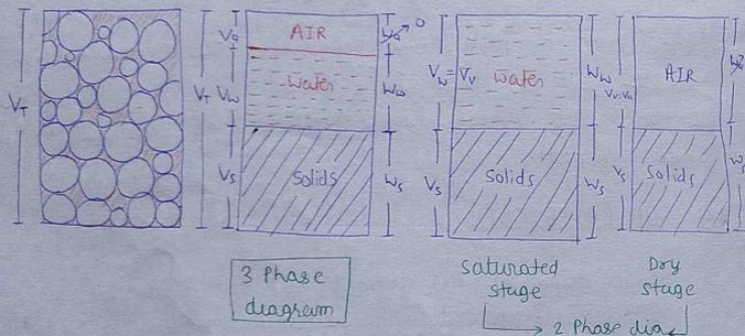
\* Soil may contain solid, liquid or Air in the mix form. Separate Representation of these Phases is termed as Phase diagram
