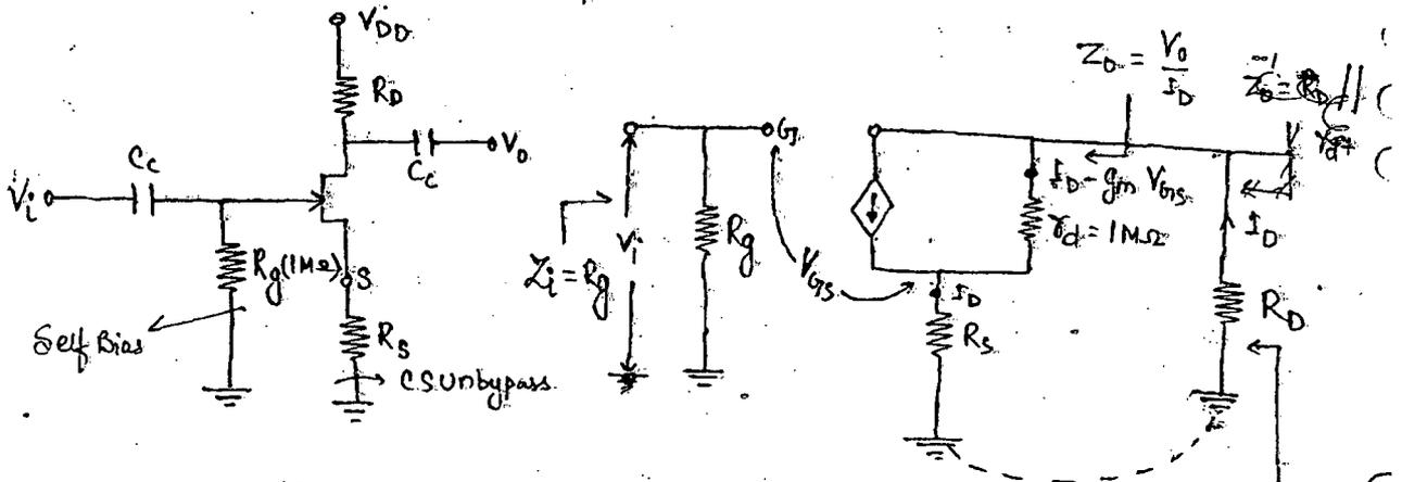
$$V_o = (I_D - g_m V_{GS}) r_d + I_D R_D$$
