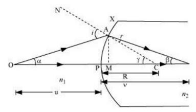
Let a spherical refracting surface XY separate a rarer medium of refractive index  $\ensuremath{n_1}$  from a denser medium of refractive index  $\ensuremath{n_2}.$  Let P be the pole, C be the centre and R = PC be the radius of curvature of this surface.
