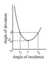
If the angle of incidence is increased gradually, then the angle of deviation first decreases, attains a minimum value  $(\delta_m)$ , and then again starts increasing. When angle of deviation is minimum, the prism is said to be placed in the minimum deviation position.
