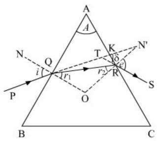
The angles of incidence and refraction at first face AB are  $\angle i$  and  $\angle r_1$
