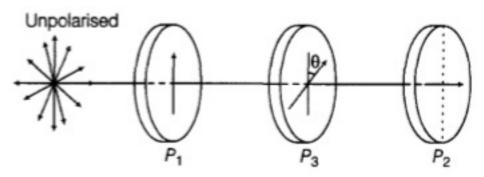
Let  $I_0$  be the intensity of polarised light after passing through the first polariser  $P_1$ . If  $\theta$  is the angle between the axes of  $P_1$  and  $P_3$ , then the intensity of the polarised light after passing through  $P_3$  will be  $I=I_0\cos^2\theta$ . As,  $P_1$  and  $P_2$  are crossed, the angle between the axes of  $P_1$  and  $P_2$  becomes 90°.
