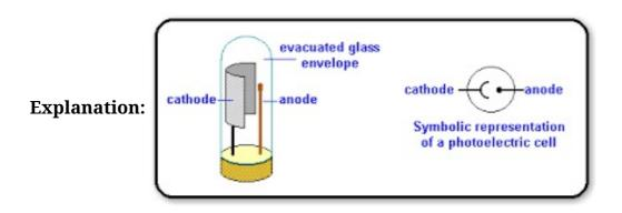
A photo cell is a device which converts light energy into electric energy.
