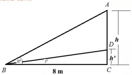
Consider the triangle  $\triangle ABC$ , AB is the hypotenuse, AC is the perpendicular and BC is the base. To find distance x follow the process. The depression angle is  $\angle B = 20^{\circ}$ ,  $\angle DBC = 5^{\circ}$
