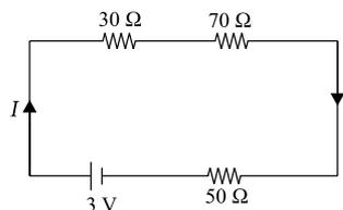
Net resistance of the circuit,  $R_N = 30 \Omega + 70 \Omega + 50 \Omega = 150 \Omega$
