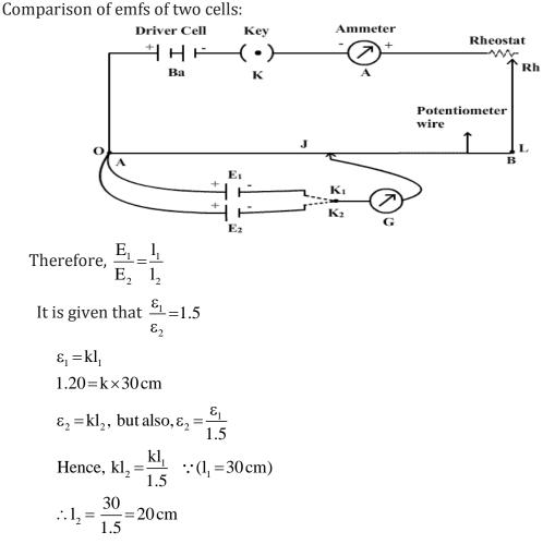
So, the difference in the balancing length of the potentiometer wire in the two cases will be:  $l_1 - l_2 = (30 - 20) = 10$  cm
