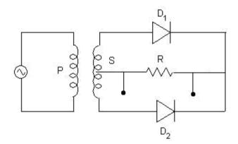
In the figure, P is the primary coil and S is the secondary coil of the transformer.  $D_1$  and  $D_2$  are the diodes which are connected to the secondary coil of the transformer. The load R, across which output voltage is obtained, is connected to a mid point on secondary coil.
