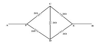
The circuit corresponds to a balanced Wheatstone bridge, and therefore no current flows in the arm CD.
