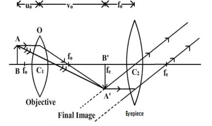
If  $m_o$  and  $m_e$  be the magnification produced by the objective lens and eye lens respectively, then the total magnifying power of microscope is  $m = m_o x m_e$ .
