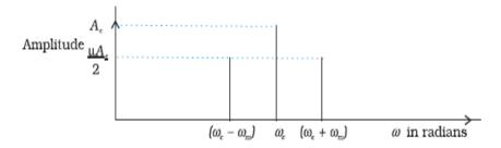
Here,  $A_c$  is the amplitude of carrier wave of frequency  $\omega_c$  and  $\omega_m$  is the frequency of modulating signal wave.  $\mu$  is the modulation index.
