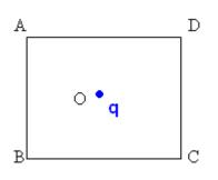
Work done: W =q (V<sub>c</sub> - V<sub>A</sub>) W =  $\frac{qQ}{4\pi\varepsilon_o} \left[ \frac{1}{OA} - \frac{1}{OC} \right]$ As, OA = OC, so W=0
