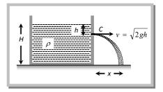
Let us find the velocity with which liquid comes out of a hole at a depth h below the liquid surface.
