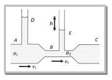
If  $P_A$  is pressure at A and  $P_B$  is pressure at B,  $P_A - P_B = h\rho g [h : difference of heights of liquids of density <math>\rho$  in vertical tubes]
