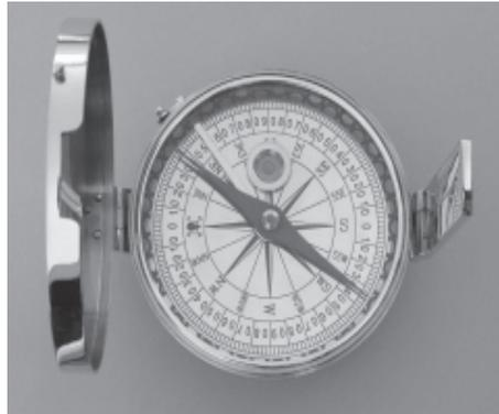
**Fig. 3.3:** Prismatic Compass
