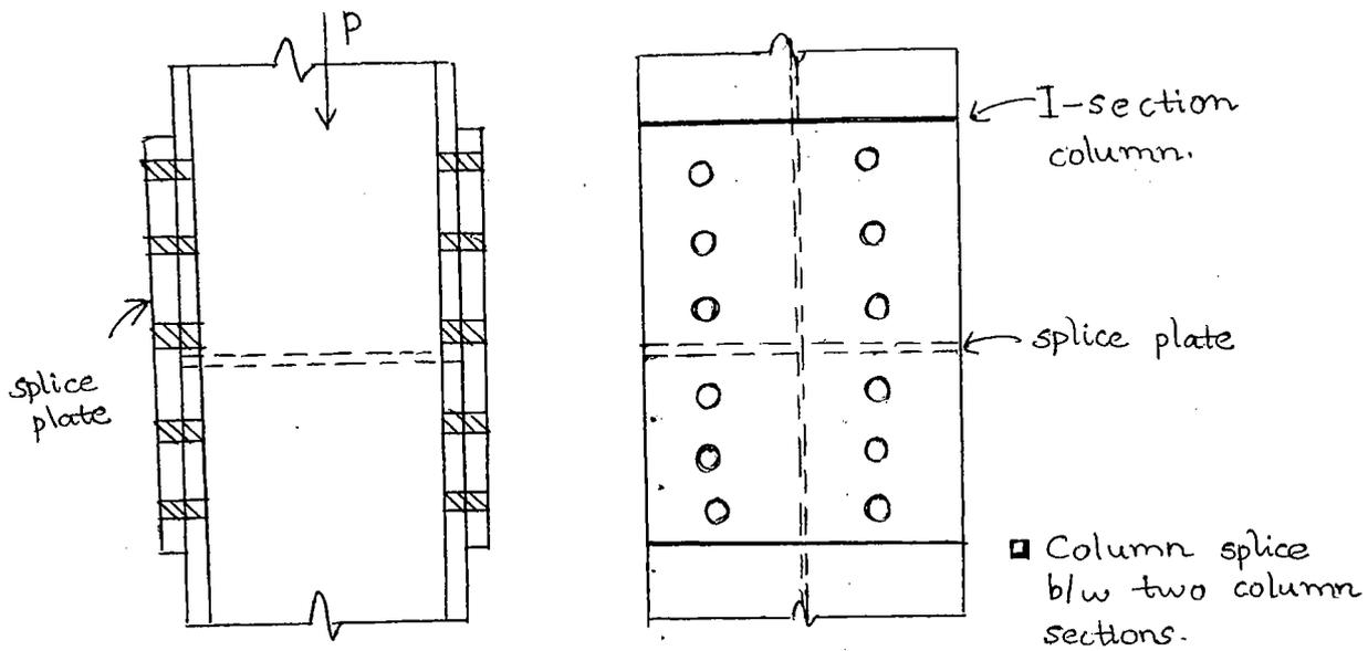
If end of a column is machined or milled, theoretically no connecting system is required. But in practise, splice must be designed for 50% factored column load.
