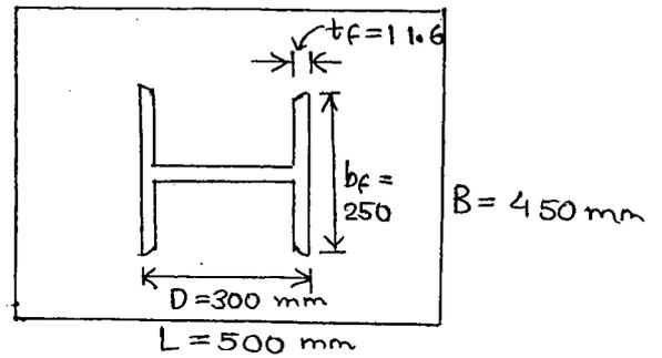
Thickness of base plate,  $t_s = \sqrt{\frac{2.5 w (a^2 - 0.3b^2) \gamma_{mo}}{f_y}}$
