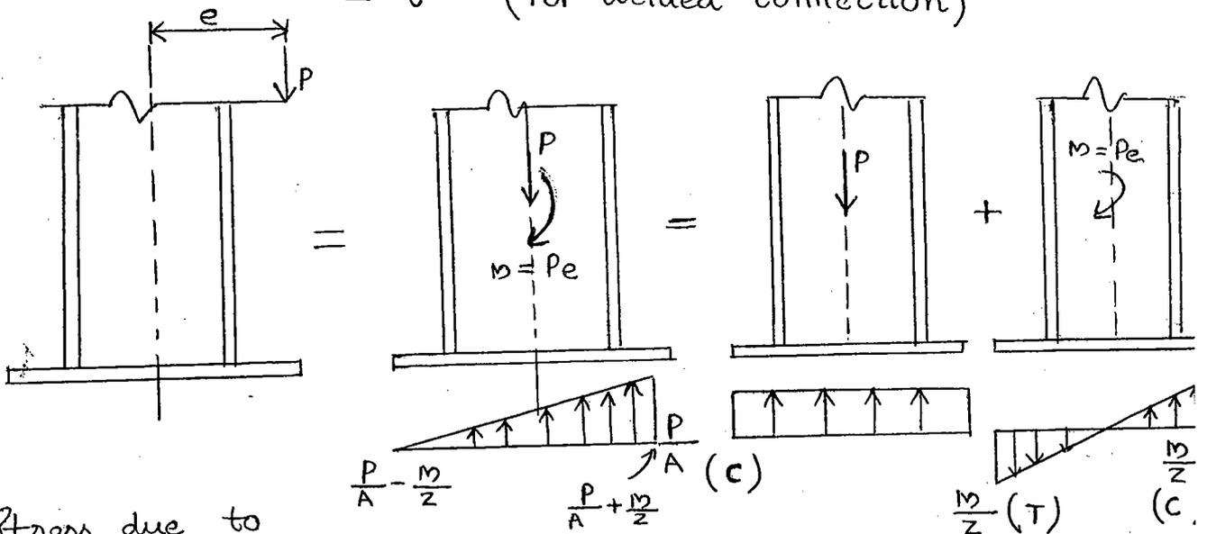
Stress due to direct axial load  $= \frac{P}{A} = \frac{P}{L \times B}$  (compression).
