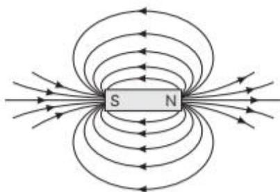
The term "uniform magnetic field" refers to an area or space with a consistent magnetic field throughout. Non-uniform magnetic field is the term used to describe the magnetic field that is different in strength and direction at every location in space.
