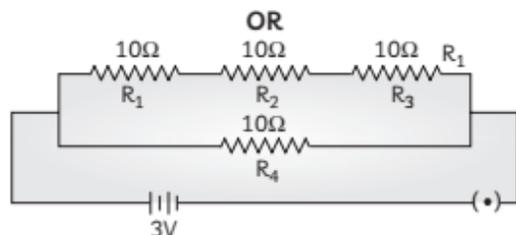
Resultant resistance of  $R_1$ ,  $R_2$  and  $R_3$ :  $R' = R_1 + R_2 + R_3 = 10 + 10 + 10 = 30\Omega$ .
