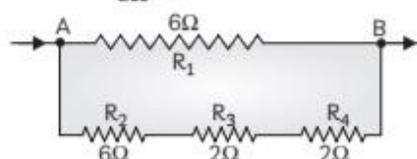
$R_2, R_3, R_4$  are in series and have resultant resistance  $R'$
