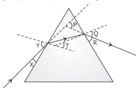
In this diagram, the angles of incidence, emergence, and deviation are, respectively:
