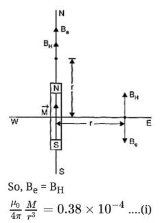
(since the dip angle (s) is zero, therefore,  $B_v = 0$  and the horizontal component of the earth's field equals the field itself)
