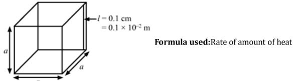
flowing or heat current is given as:  $\frac{\Delta \theta}{\Delta t} = K \times \frac{A\Delta T}{x}$  Here,  $\Delta \theta$  is the amount of heat transferred,  $\Delta T$  is the temperature difference, K is the thermal conductivity of the material, A is the area of cross section of the material and x is the thickness or
