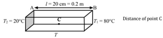
from left end: x' = 11cm = 0.11 mFormula used:(b)Rate of amount of heat flowing or heat current is given as:  $\frac{\Delta \theta}{\Delta t} = K \times \frac{A\Delta T}{x}$  Here,  $\Delta \theta$  is the amount of heat
