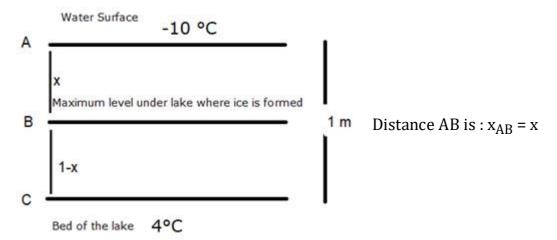
m Distance CB is :  $x_{CB}$  = (1-x) m Formula used: Rate of amount of heat flowing or heat current is given as:  $\frac{\Delta \theta}{\Delta t} = K \times \frac{A\Delta T}{X}$  Here,  $\Delta \theta$  is the amount of heat transferred,
