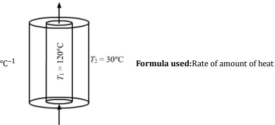
flowing or heat current is given as:  $\frac{\Delta \theta}{\Delta t} = K \times \frac{A\Delta T}{x}$  Here,  $\Delta \theta$  is the amount of heat transferred,  $\Delta T$  is the temperature difference, K is the thermal conductivity of the material, K is the area of cross section of the material and K is the thickness or length of the material. Consider an element dx at a distance of K from the center
