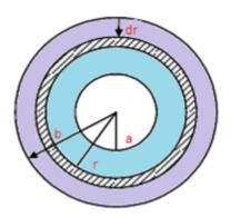
Let-Radius of the inner sphere = aRadius of the outer sphere = b
