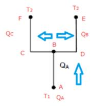
Let  $Q_A$ ,  $Q_C$  and  $Q_B$  be the heat currents, i.e. rate of flow of heat per unit time in AB, BCE and BDF, respectively.
