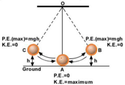
At the points B and C, the pendulum bob is at its maximum height, so its potential energy is maximum and kinetic energy is zero. In this way the total mechanical energy remains constant. At the point A, the pendulum bob is at its lowest point, total potential energy is converted into kinetic energy. Now the kinetic energy is maximum and potential energy is zero. Once again the total mechanical energy remains constant.
