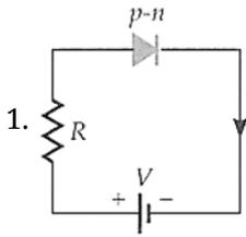
The figure shows a forward-biased p-n junction diode in which p-side is connected to the +ve terminal and n-side is connected to the -ve terminal of the battery and shows its voltage-current graph.
