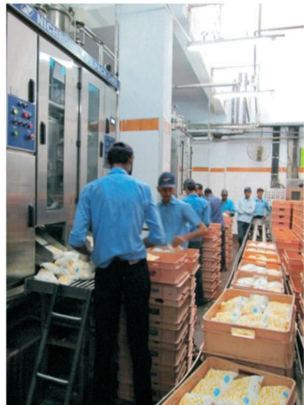
Fig.14.2. Packaging of pasteurized milk in pouches
