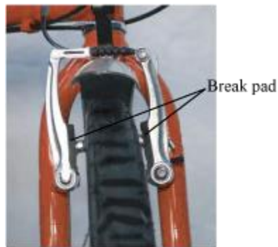
Before the application of breaks
