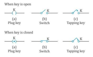
When a key is closed, i.e. the plug is inserted, the circuit is called a **closed circuit**.
