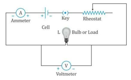
**Functions of Various Components in a Circuit**
