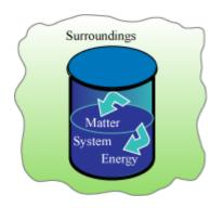
Example – Presence of reactants in a thermos flask or any other closed insulated vessel
