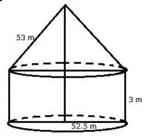
For the cylindrical portion, we have radius = 52.5 m and height = 3 m For the conical portion, we have radius = 52.5 m And slant height = 53 m Area of canvas = 2rh + rl = r(2h + l)
