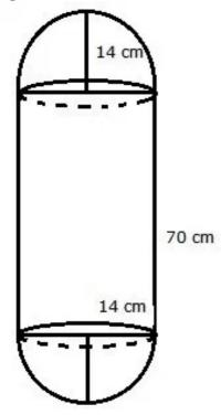
Radius of each hemispherical end =  $\frac{28}{2}$  = 14 cm Height of each hemispherical part = Its Radius Height of cylindrical part =  $(98 - 2 \times 14) = 70$  cm Area of surface to be polished = 2(curved surface area of hemisphere) + (curved surface area of cylinder)
