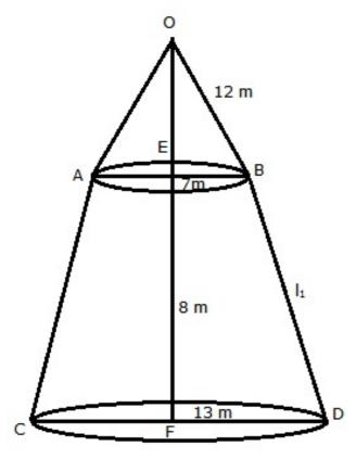
ABCD is the frustum in which upper and lower radii are EB = 7 m and FD = 13 m Height of frustum = 8 m Slant height  $l_1$  of frustum
