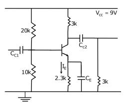
80.The value of DC current  $I_E$  is<br/>(A) 1mA(B) 2mA(C) 5mA(D) 10mA81.The mid-band voltage gain of the amplifier is approximately<br/>(A) -180(B) -120(C) -90(D) -60
