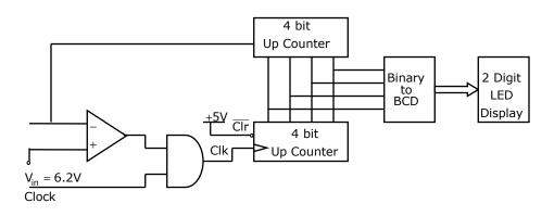
82. The stable reading of the LED display is(A) 06 (B) 07 (C) 12 (D)13
