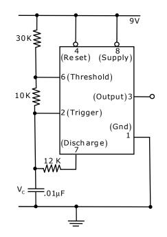
The voltage V<sub>c</sub> across the capacitor varies between (A) 3V to 5V (B) 3V to 6V (C) 3.6V to 6V (D) 3.6V to 5V
