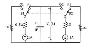
Assume that the capacitor has zero initial charge. Given that u(t) is a unit step function, the voltage  $V_c(t)$  across the capacitor is given be
