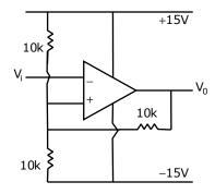
A triangular wave which goes from -12V to 12V is applied to the inverting input of the OPAMP. Assume that the output of the OPAMP sings from +15V to -15V. The voltage at the non-inverting input switches between
