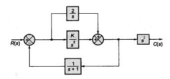
If the poles location for this system is as shown in figure below, then the value of *K* is \_\_\_\_\_
