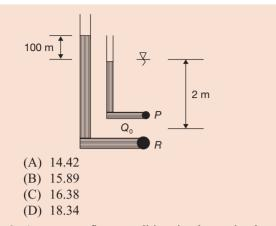
6. A seepage flow condition is shown in the figure. The saturated unit weight of the soil  $\gamma_{sat} = 18 \text{ kN/m^3}$ . Using unit weight of water,  $\gamma_w = 9.81 \text{ kN/m^3}$ , the
