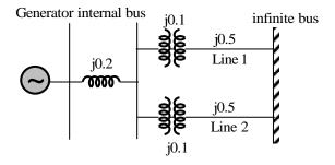
The p.u. reactances of different components in the system are also shown in the figure. The infinite bus voltage magnitude is 1.0p.u.
