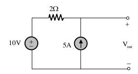
The voltage  $\left(V_{\mbox{\tiny out}}\right)$  across the current source, in volts, is
