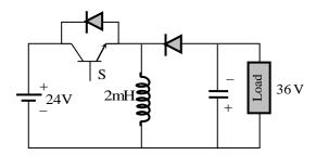
It is operated at 20kHz with an inductor of 2 mH and output capacitor of 1000  $\mu$ F. All devices are considered to be ideal. The peak voltage across the solid-state switch (S), in volt, is \_\_\_\_\_.
