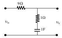
the frequency (in rad/s) at which the maximum phase lag occurs is.\_\_\_\_\_.
