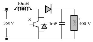
Considering continuous inductor current, the rms current in the solid state switch (S), in ampere, is \_\_\_\_\_\_.
