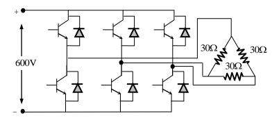
If it is fed from a 600V battery, with  $180^{\circ}$  conduction of solid-state devices, the power consumed by the load, in kW, is \_\_\_\_\_.
