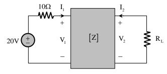
The average power delivered to  $R_L = 20\Omega$ , in watts, is \_\_\_\_\_.
