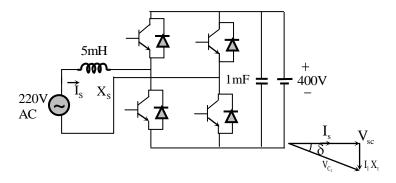
All devices are ideal. It is used to charge a battery at 400V with power of 5kW from a source sinusoidal AC mains at unity p.f. If its ac side interfacing inductor is 5mH and the switches are operated at 20kHz, then the phase shift ( $\delta$ ) between AC mains voltage ( $V_s$ ) and fundamental AC rms VSC voltage ( $V_{Cl}$ ), in degree, is
