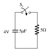
The charge (in  $\mu$ C) lost by the capacitor from  $t = 25\mu$ s to  $t = 100 \,\mu$ s is \_\_\_\_\_.
