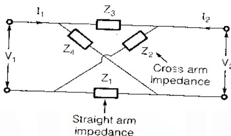
1. A lattice network is said to be symmetrical if the two straight arm impedances are equal i.e.  $Z_1 = Z_3$ .
