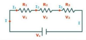
The current passing through the individual resistance is same and its equal to magnitude of current that comes from the battery.
