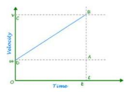
The body has an initial velocity u at point A and then its velocity changes at a uniform rate from A to B in time t. In other words, there is a uniform acceleration 'a' from A to B, and after time t its final velocity becomes 'v' which is equal to BC in the graph. The time t is represented by OC. To complete the figure, we draw the perpendicular CB from point C, and draw AD parallel to OC. BE is the perpendicular from point B to OE.
