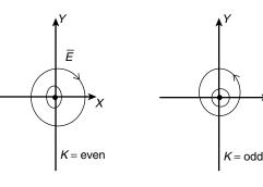
k = even close wise circular Polarization (Left circular Polarization) k = odd Counter clockwise circular Polarization (Right circular polarization)
