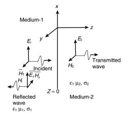
Assuming the electric field does not undergo any variation and the wave is travelling in z direction. Then, the fields are shown in above figure.
