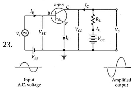
**Condition:** For a transistor to act as an amplifier, it must be operated close to the centre of its active region.
