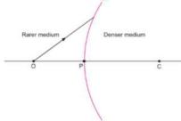
Complete the path of an incident ray of light, showing the formation of a real image. Hence derive the relation connecting object distance u, image distance v, radius of curvature R, and the refractive indices n<sub>1</sub> and n<sub>2</sub> of the two media.
