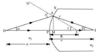
Let a spherical refracting surface XY separate a rarer medium of refractive index  $n_1$  from a denser medium of refractive index  $n_2$ . Let P be the pole, C be the centre and R = PC be the radius of curvature of this surface.
