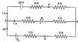
ii. If in the circuit, the polarity of the battery E<sub>1</sub>, be reversed, what will be the potential difference between A and B?
