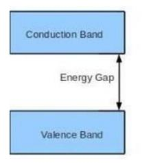
In this case, there is large forbidden gap approx. 5ev upon the nature of the crystal. Electrons, however heated, find it practically impossible to jump this gap and thus never reach the conduction band. Thus, electrical conduction is not possible through an insulator, normally carbon is a conductor but the same carbon as diamond, with the energy gap of 7ev is perfect insulator.
