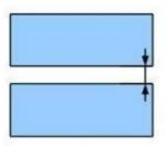
In above figure. There is overlapping of valence and conduction bands. This is because the lowest levels in the conduction band need less energy than the highest levels in the valence band and electrons in the valence field, contribute to electrical conduction.
