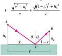
To minimize the time we set the derivative of the time with respect to x equal to zero. We also use the definition of the sine as opposite side over hypotenous to relate the lengths to the angles of incident and reflection.
