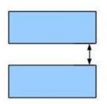
In this class of crystals the two energy bands are distinctly separate with no overlapping. The forbidden gap and reach the conduction band. Therefore, the substance is an insulator. But at room temperature, some valence electrons acquire thermal energy greater then the gap and move to the conduction band where they are free to move influence of even a weak electric field.
