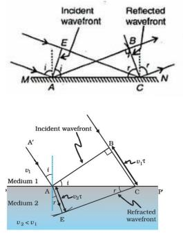
We can see a ray of light is incident on this surface and another ray which is parallel to this ray is also incident on this surface. As these rays are incident from the surface, so we call it incident ray.
