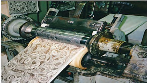
● Screen Printing : In the early 20 th Century the modern process of screen printing arrived, although it is thought that screen printing dates back much further than this. This process is similar to that of Stencil Printing but the scale is much larger. It involves making a pattern on a screen of porous mesh-which was traditionally made of silk. It can be of two types : ● Rotary Screen Printing: Where a roller is used to pull ink over the stencil which is in turn forced through the mesh and onto the fabric.
