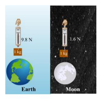
Suppose a body of mass 1000 kg is placed on Earth's surface and then on the surface of the moon. The mass of the body will remain the same at both places, but it will have different weights (9800 N on Earth and 1600 N on the moon).
