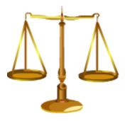
A beam balance is also used for measuring the mass of a body. It does so by comparing the mass of the body with a given standard mass.
