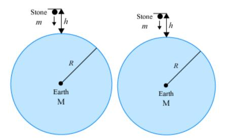
Therefore, the man must go  $(R+h) = (6.4 \times 10^6 + 2.65 \times 10^6 = 9.05 \times 10^6)$  m far from Earth's centre so as to weigh 40 N.
