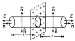
Electric flux through both the surfaces are positive as Electric field lines are originating from them and net electric flux will be the sum of these individual fluxes.
