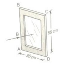
The window is hinged along the edge AB. When the window is closed, the horizontal component of the earth's magnetic field of flux density  $1.8\times10^{-4}$ T, is normal to the window.
