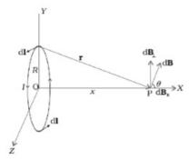
According to Biot Savart Law, the magnitude dB of the magnetic field due to dl is given by,
