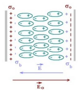
This reduces the electric field in between the plates. The potential is also reduced. Maximum potential is dependent on the charge on the plates. As the charge remains constant, the presence of the dielectric decreases the maximum potential between the plates.
